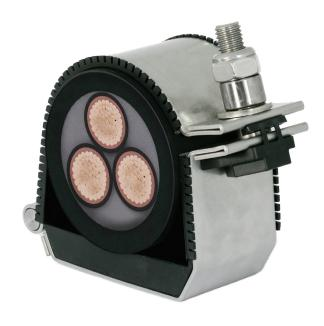
The SHDSS cable cleat range consists of metallic cable cleats which have been designed, constructed, and tested in accordance with the International Standard IEC 61914: Cable cleats for electrical installations.
